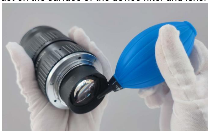
Figure 2-1 Cleaning by Rubber Dust Air Blower
